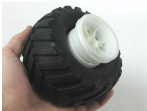
Figure 4.1 Inserting the tire in the rim
